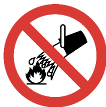
Extinguishing with water is prohibited
